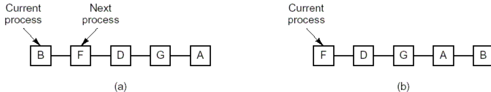
Figure 2-22. Round robin scheduling. (a) The list of runnable processes. (b) The list of runnable processes after B uses up its quantum.
